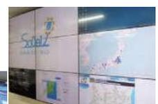
Configuring a large display made of 9 59cm x 105cm panels. The status of all of Mega Solar's electricity generation systems countrywide can be observed easily
